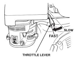
Figure 12. Throttle Lever
